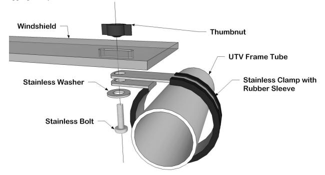
10. If using the Aero-Vent Lexan windshield with one of Over Armour Cab Enclosures the top brace will be used to seal the top of the enclosure to the top of the windshield. After installing the enclosure over the windshield take a small knife and cut an x into the canvas where each hole is across the top of the windshield. Then install the brace as shown in the picture below.
