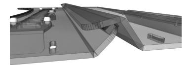
9. The diagram below shows the proper placement sequence of the hardware. Use the 1" bolts for this application. Install each one loosely at first; after you have centered the windshield and are satisfied with exact placement, then you may snug the thumbnuts appropriately.
