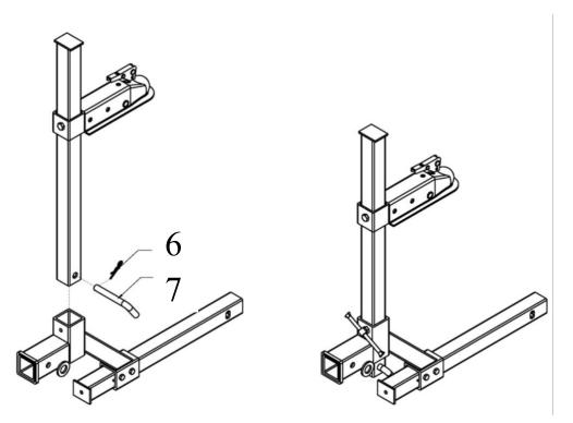
NOTE: In some cases, the coupler comes with a bolt installed for shipping purposes only. This must be removed before the unit will operate properly! Be sure to adjust the coupler nut to the hitch ball size before operation!!!!
