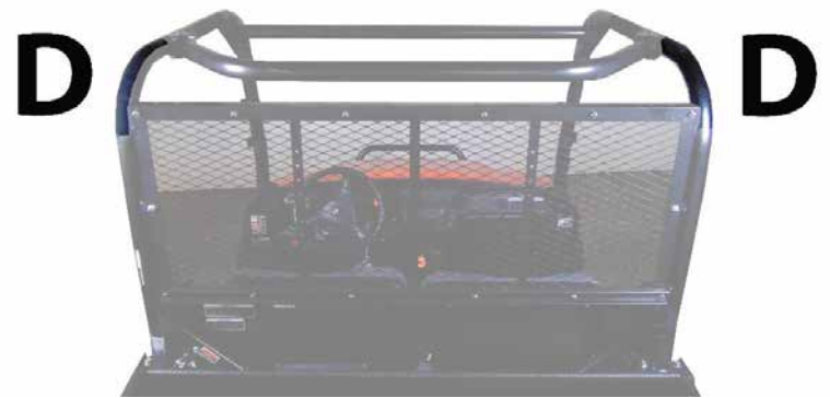
Figure 4: Shows placement of 21" Velcro strips D. Start strip at the metal bracket on the top and attach to the curve down to the metal grate.
