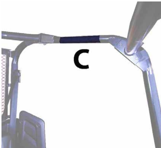
Figure 3: Shows placement of 12" Velcro strips C. Attach soft Velcro on the top of the door, pull the door around the top so that the seam lines up to the middle of the roll bar.
