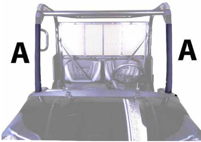
Figure 1: Shows placement of 26" Velcro strip A. The tabs on the front of your doors will wrap around the front of the roll bar and attach to the Velcro strip. The detachable straps will stick to this strip.
